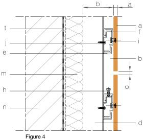
Figure 4 Horizontal panel joint
