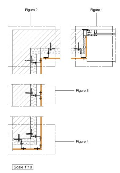
This drawing indicates a typical fixing arrangement on a metal supporting structure. Please contact your Formica Group representative for other possibilities.
