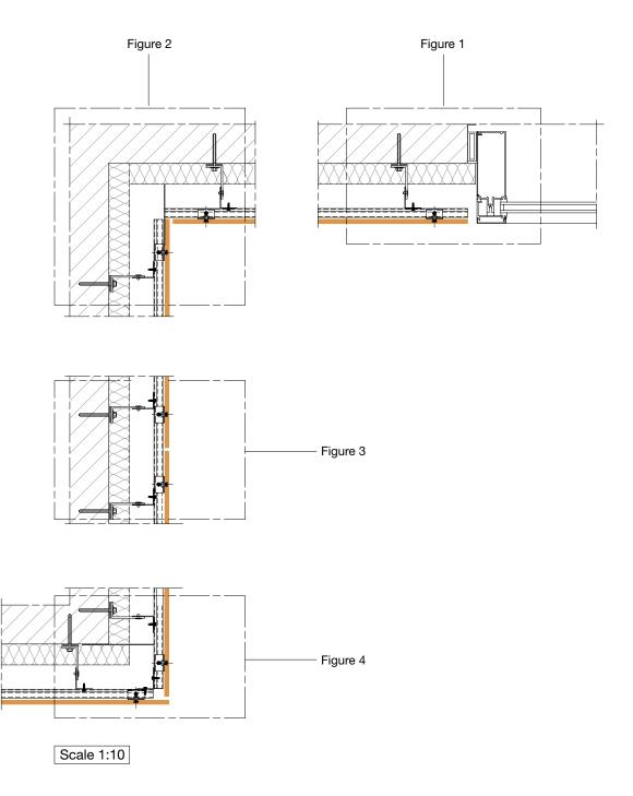
This drawing indicates a typical fixing arrangement on a metal supporting structure. Please contact your Formica Group representative for other possibilities.
