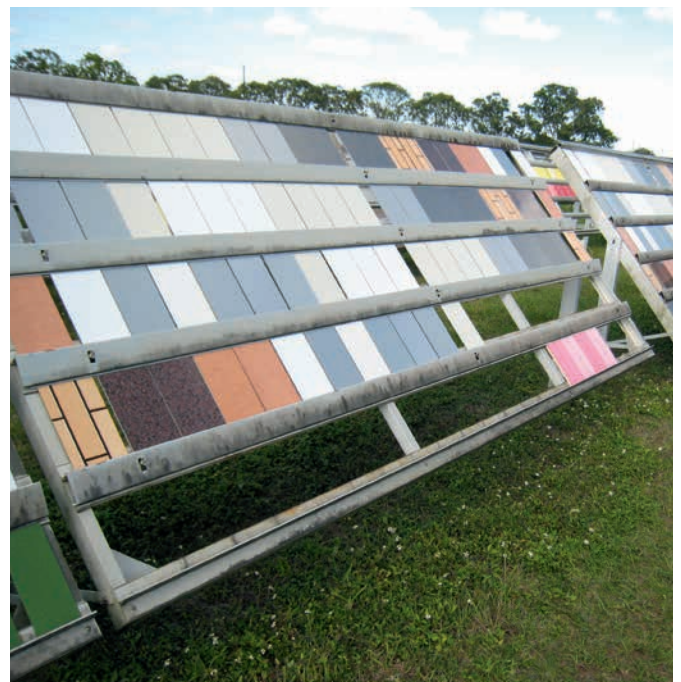
Natural exposure test in Florida, USA
