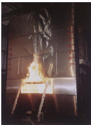
Example of fire test for exterior
